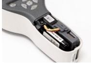
5. Put the new battery in the same position and attach the connector to its socket.
