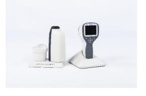
7. Camera will not automatically power up in the cradle without the charger. User needs to press the power button.
