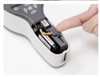
4. Remove the old battery by placing your fingernail underneath the connector's edge and lifting the connector and the battery out of their sockets to disconnect the battery.
