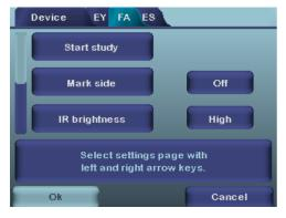
Arrow keys change values in the menu. Active value is indicated with light blue color. Changed values are saved by using left soft key ("Ok") and cancelled by pressing right soft key ("Cancel"). Some values are confirmed by pressing the Middle key.
