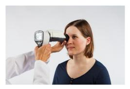
9. Still image is captured by pressing the shutter button all the way down. If half-press capture is enabled, still image can be captured by pressing shutter button halfway down. Taken image is displayed on screen until user clears the image by pressing shutter button, left or right soft key.
